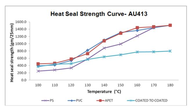
Sealing condition: Sealed at 420 N, 1 second
