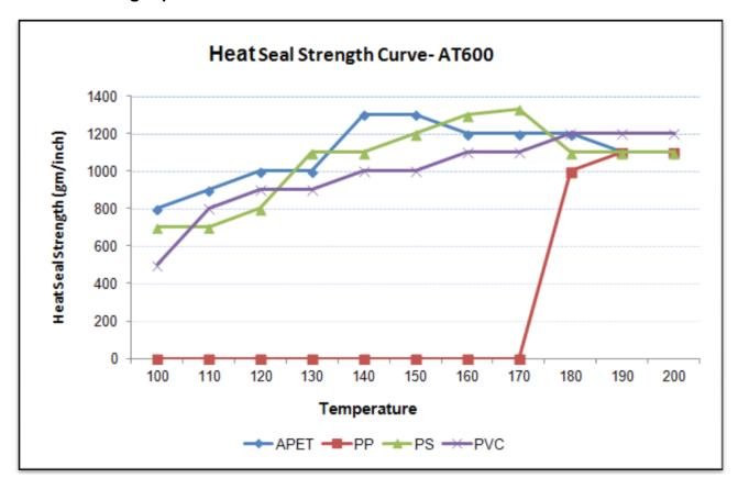
Sealing condition: Sealed at 420 N, 1 second
